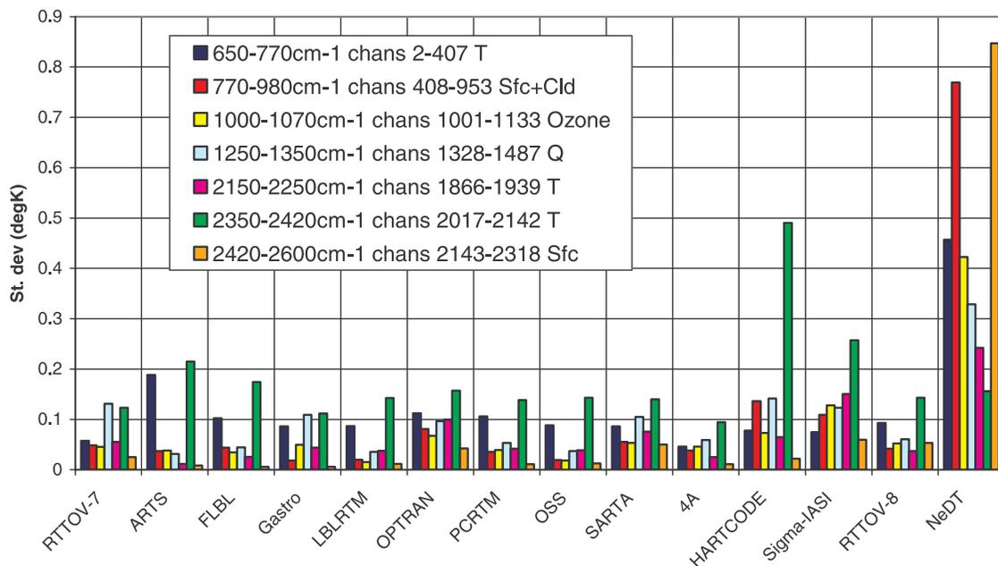
**Figure 4.** A histogram of the RT model nadir view differences from RFM for different spectral regions. The columns on the far right give the AIRS instrument noise for a 250 K brightness temperature scene.
